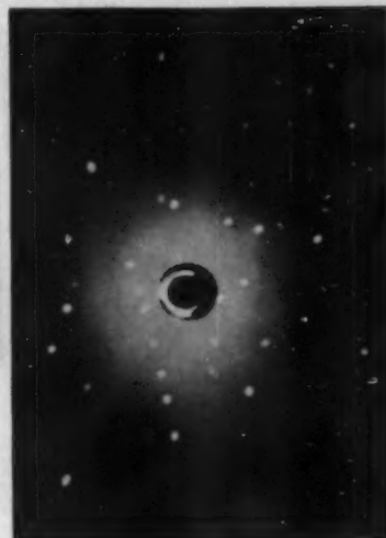
FIG. 4. Laue back-reflection x-ray pattern of single-crystal vapor-deposited Ge layer after removal from substrate.
